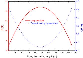
Figure 8. Magnetic field and current sharing temperature at 56 kA along the cooling length of the A1 channel.
