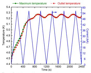
Figure 12. Maximum cable temperature, outlet temperature and current evolution as functions of time for the A1 channel.
