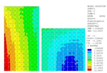
Figure 2. Magnetic field distribution of the superconducting magnet at 56 kA (Unit: T).
