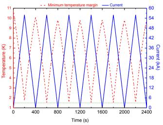
Figure 10. Minimum temperature margin and current evolution as functions of time for the A1 channel.
