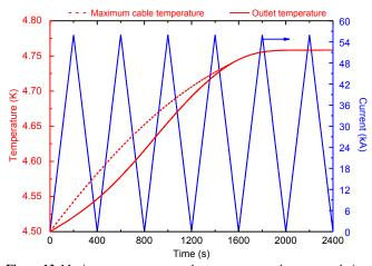
Figure 13. Maximum temperature, outlet temperature and current evolution as functions of time for the B1 channel.
