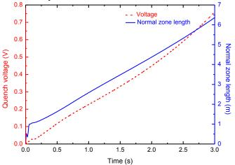
Figure 15. Normal zone length and quench voltage evolution as functions of time for the A1 channel.
