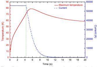
Figure 17. Hot spot temperature evolution as a function of time for the A1 channel.
