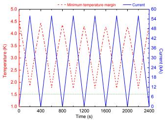
Figure 11. Minimum temperature margin and current evolution as functions of time for the B1 channel.
