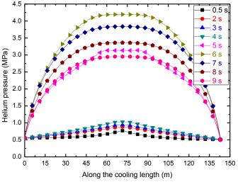
Figure 20. Helium pressure evolution along the cooling length as a function of time for the A1 channel.
