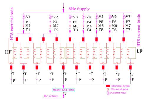
Figure 7. Cooling circuit of the superconducting magnet.
