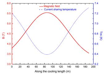
Figure 9. Magnetic field and current sharing temperature at 56 kA along the cooling length of the B1 channel.
