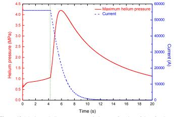
Figure 19. Maximum helium pressure evolution as a function of time for the A1 channel.
