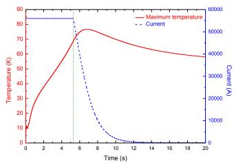
Figure 21. Hot spot temperature evolution as a function of time for the B1 channel.
