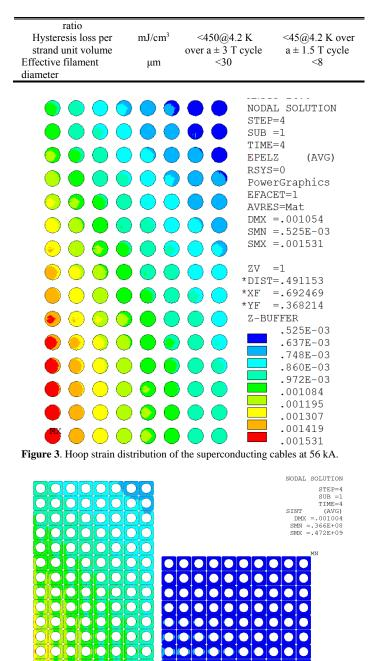
C  $\cap$ 1 ( $\cap$ 0  $\cap$ .327E+09 .133E+09 .230E+09 .849E+08 .182E+09 .375E+09 .472E+09 Figure 4. Tresca stress distribution in the jacket of the superconducting
