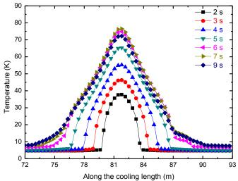
Figure 23. Cable temperature evolution along the cooling length as a function of time for the B1 channel.
