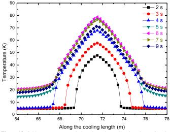
Figure 18. Cable temperature evolution along the cooling length as a function of time for the A1 channel.
