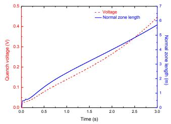
Figure 16. Normal zone length and quench voltage evolution as functions of time for the B1 channel.
