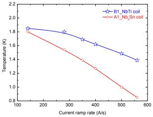
Figure 14. The lowest value of the minimum temperature margin vs current ramp rate for cyclic operation.
