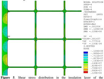
**Figure 5.** Shear stress distribution in the insulation layer of the superconducting magnet (Unit: Pa).
