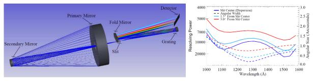
Figure 7. At left, we show a raytrace of the SISTINE payload. The telescope is a 0.5-m primary Cassegrain design. Ar right, we show performance projections for SISTINE. The solid lines show the predicted spectral resolving power (left axis) and the dotted lines show the imaging performance as a function of wavelengths and field position (in arcsec, right axis).
