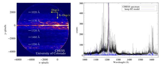
Figure 9. Calibration data from the CHESS instrument (*left*), demonstrating R ≈ 70,000; the orders are separated top-to-bottom, each order has 5 – 7 Å of free spectral range. The extracted one-dimensional spectrum is shown at right (Hoadley et al. 2014). A grating mount shift during launch on 36.285 reduced the instrumental resolution and efficiency (see Figure 14 below).
