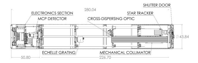
Figure 5. Schematic of the spectrograph section of CHESS. Labeled are relevant disk structures and optical components.
