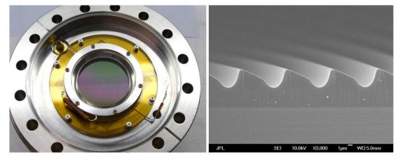
Figure 6. New hardware for the CHESS-2 payload: (*left*) the 40mm cross-strip anode MCP detector following the deposition of a new photocathode at Sensor Sciences. (*right*) Scanning Electron Microscope cross-sectional image of the electron-beam etched echelle grating produced at JPL. The 100 groove mm<sup>-1</sup> design enables higher groove efficiency, but at the cost of continuous spectral coverage at  $\lambda > 1300$  Å.
