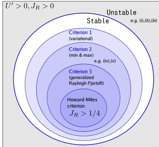
Figure 3: Venn diagram of sufficient stability criteria
