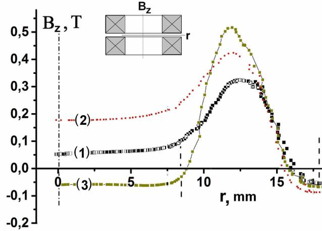
Fig. 3. The radial field distribution  $B_z(r)$  at the different conditions: (1) – after the single pulse of  $\mu_0 H_a = 0.9$  T; (2) – after 10 pulses with peak field  $\mu_0 H_a = 0.9$  T; (3) after the flux jump  $\mu_0 H_a = 2.0$  T. The vertical dotted lines corresponds to the inner and outer annuli radii.
