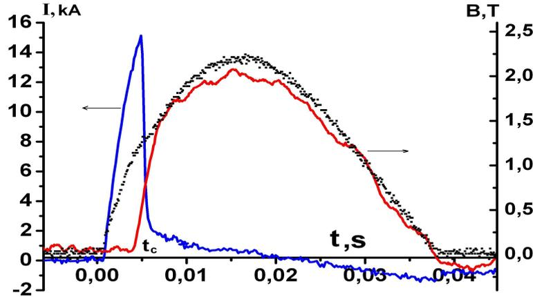
Fig. 2. The evolution of the current and the field. Left axis – the current in annuli –  $I(t)$ . Right axis – the external field (dots) and the field in the hole (solid curve).
