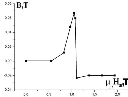
Fig. 1. The trapped field in the center of the annuli as a function of the pulse field amplitude.
