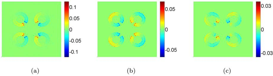
Fig. 4: Surface charge distribution at the angle of  $45^\circ$  of (a) $LC$  mode ( $N = 1$ ), (b)plasmon mode ( $N = 2$ ) and (c)quadrupole mode ( $N = 3$ ).
