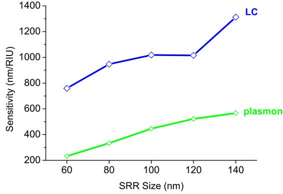
Fig. 9: Simulated sensitivity for the quad-supercell metamaterials with different sizes.
