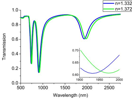
Fig. 8: The transmission spectra for the quad-supercell metamaterials by changing 100 nm thick cover layer filled with water ( $n = 1.332$ ) to 25% aqueous glucose solution ( $n = 1.372$ ). Inset: enlarged figure of the shift of the transmission dip.
