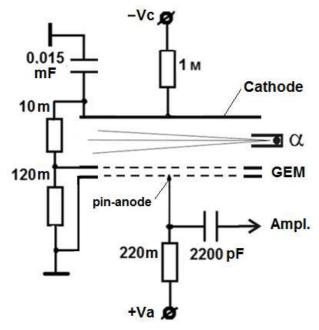
Figure 1. GEM+pin-anode.
