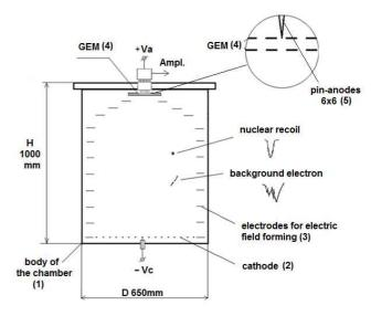
Figure 3. The chamber with  $Ne+10\%H_2$  filling.
