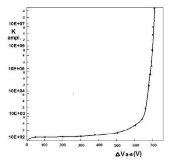
Figure 2. The dependence of  $K_{ampl.}$  on potential difference between the pin-anode and GEM,  $K_{ampl}=Q_{ampl}/Q_{ioniz}$ , where  $Q_{ampl}$ -the charge detected,  $Q_{ioniz}$ -the ionization charge.
