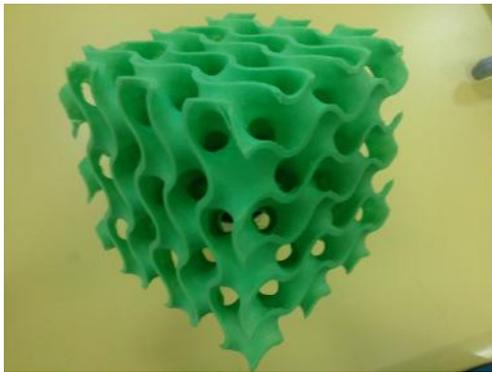
“Gyroid structure” for photonic crystals
