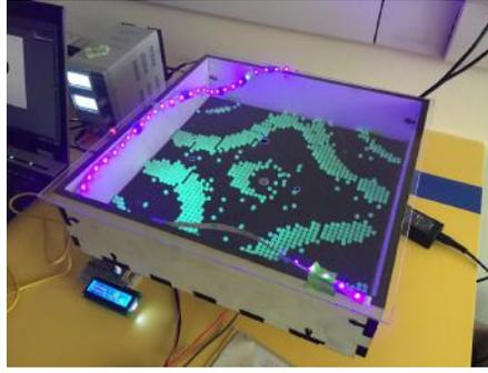
Chladni figures, with the peculiarity of replacing sand with larger spheres moving on a 3D printed net of different geometries and under frequencies adjusted via an Arduino
