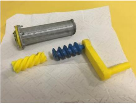
Moineau+Auger pump for volumetric flow proportional to the rotation rate
