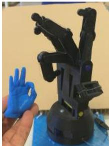
First prototype for a “Voice-Controlled Artificial Handspeak System” –an automated translator for communication with the deaf to help reduce language barriers [13].
