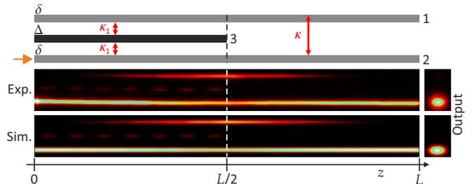
FIG. 3. Interferometric phase verification. The three-site structure is superseded by a regular coupler at  $z = L/2$ . The sign reversal of the coupling leads to refocussing in the injection channel. The parameters are as before, except  $\Delta = 61\kappa$ .
