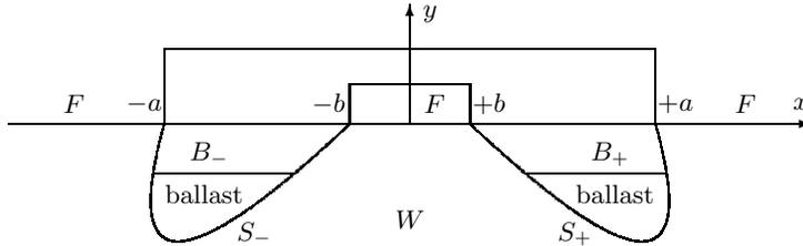
Figure 1: A definition sketch of the cylinder cross-section with immersed parts denoted by  $B_-$  and  $B_+$ ; their wetted boundaries are  $S_-$  and  $S_+$  respectively. The cross-section of the infinitely thin layer of the brash ice covering the free surface is denoted by  $F$ ; it consists of three parts two of which lie on the  $x$ -axis outside  $|x| > a$  and the third one is between  $x = -b$  and  $x = +b$ ;  $W$  is the cross-section of the water domain.
