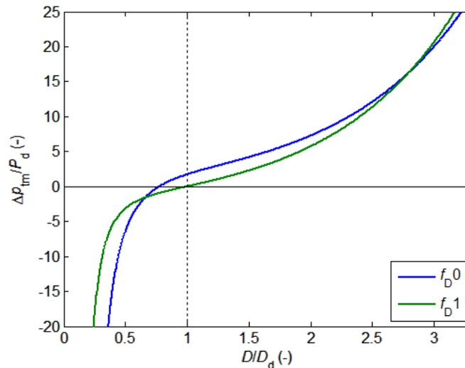
Figure 1 Comparison of the original ( $f_{D0}$ ) and revised ( $f_{D1}$ ) forms of passive constitutive relation. Lymphangion diameter is normalised by the parameter  $D_d$ ; transmural pressure is normalised by the parameter  $P_d$ . The slope of  $f_{D1}$  at  $D = D_d$  is  $4P_d/D_d$ .
