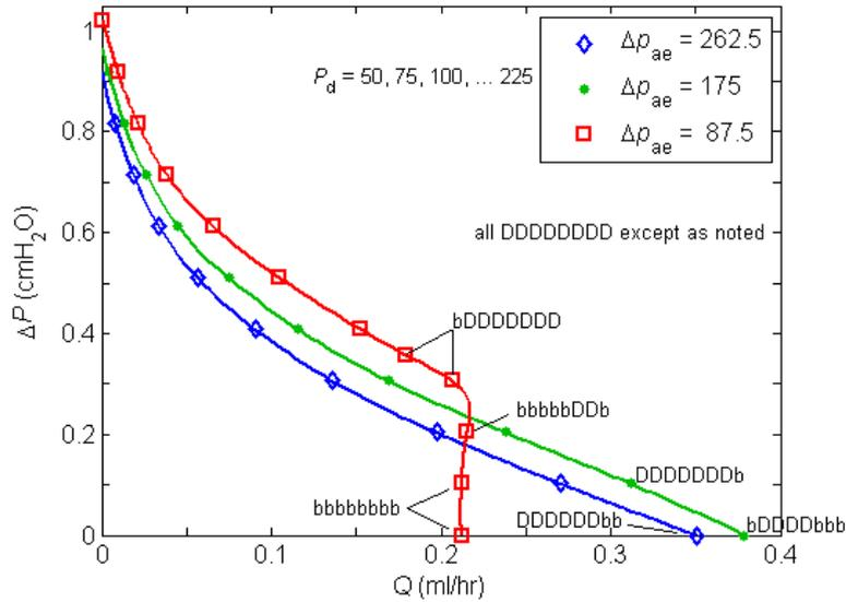
Figure 5 Pump function curves for the same  $f_{D1}$  model as above, at three levels of inlet transmural pressure  $\Delta p_{ae}$  ( $\text{dyn cm}^{-2}$ ) as indicated in the legend; all other parameters as for Fig. 3. The bD codes are explained in the caption to Fig. 3.
