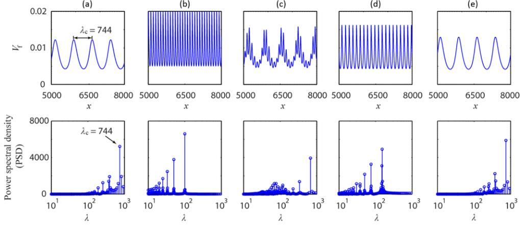
Figure 4: Simulation results of Arrhenius reaction-rate model ( $\sigma = 0.1$  and  $N = 8$ ). Upper row: history of the instantaneous flame velocity as a function of position. Lower row: PSD obtained via FFT plotted in wavelength domain for the following cases: (a) continuous, (b)  $L = 100$ ,  $\Gamma = 0.1$ , (c)  $L = 100$ ,  $\Gamma = 0.5$ , (d)  $L = 150$ ,  $\Gamma = 0.5$ , and (e)  $L = 30$ ,  $\Gamma = 0.5$ .
