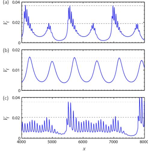
Figure 5: Simulation results of the history of the instantaneous flame velocity as a function of position with Arrhenius reaction-rate model ( $\sigma = 0.1$  and  $N = 8$ ) for the cases of  $\Gamma = 0.05$  and  $L =$  (a) 50, (b) 30, and (c) 80.
