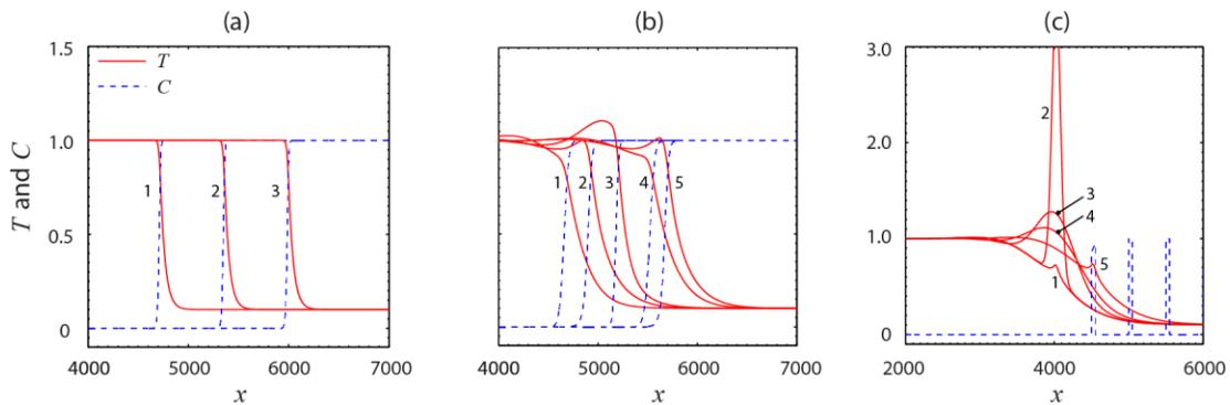
Figure 3: Sample results of Arrhenius reaction-rate model for (a) continuous, stable ( $\sigma = 0.1$ ,  $N = 6$ , and  $\Gamma = 1$ ), and (b) unstable ( $\sigma = 0.1$ ,  $N = 8$ , and  $\Gamma = 1$ ), and (c) discrete ( $\sigma = 0.1$ ,  $N = 8$ ,  $L = 500$ , and  $\Gamma = 0.1$ ) cases. The numeric labels indicate the chronological order of the snapshots of  $T$  and  $C$  profiles.
