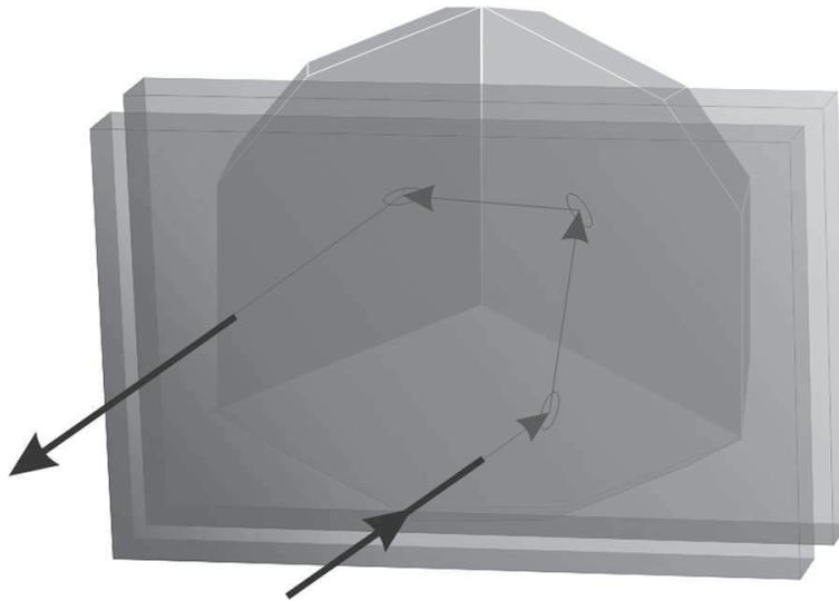
**FIGURE 2** A corner cube prism with two liquid crystal modulators mounted on top. The light passes through the liquid crystal once, bounces on the three internal surfaces of the retro-prism, and passes through the liquid crystal modulators to return in the direction of origin.
