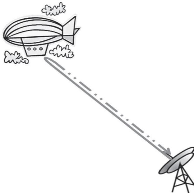
**FIGURE 1** The principle of retro-modulation: A laser beam is directed towards a cats-eye or retro-mirror, which is combined with an electro optical modulator. The retro-mirror returns the modulated beam towards the emitter, and thus an airborne laser is avoided.
