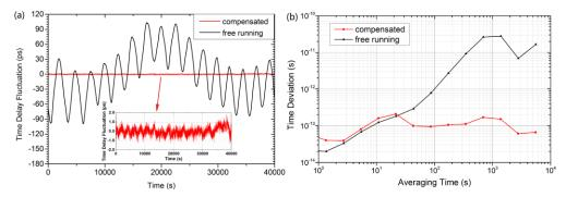
Fig. 3. Measurement results of the uncompensated and compensated system delays. (a) The system delay fluctuation. The black line is the result when the system internal fiber is running freely, showing a fluctuation of  $\pm 100 ps$ . The red line is the result with the system delay fluctuation compensated, showing a fluctuation of  $\pm 1 ps$ . (b) The time deviation of the system delay derived from the measured system delay fluctuation.
