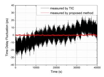
Fig. 4. Measurement results of the compensated system delay fluctuations using two methods. The black line is the result measured by TIC, showing a fluctuation of  $\pm 25 ps$ . The red line is the result measured by proposed method, showing a fluctuation of  $\pm 1 ps$ .
