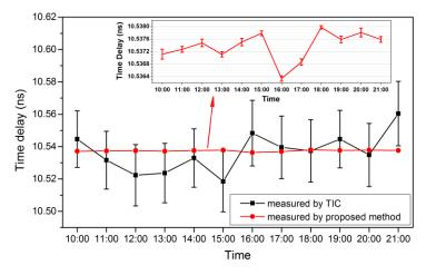
Fig. 5. FTD measurement results of a 2 m long fiber. The averaging period is 100 s. The error bar is the standard deviation of each measurement. The black line is the FTD measured by TIC, showing a long-term fluctuation of  $\pm 20 ps$  with an uncertainty of 20 ps. The red line is the FTD measured by proposed method. The long-term fluctuation is reduced to  $\pm 1 ps$  with an uncertainty below 0.2 ps.
