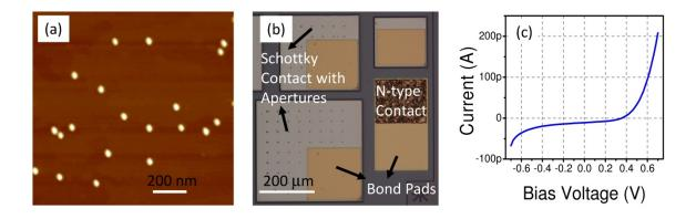
**Figure 1** (a) Atomic force microscopy image of a typical InAs quantum dot wafer with a dot density of  $10^9 \cdot \text{cm}^{-2}$ . (b) Optical microscopy image of the Schottky diode structure with arrays of small apertures to address single quantum dots. (c) A typical *I–V* curve of the Schottky diode with a mesa area of 400  $\mu$ m × 400  $\mu$ m.
