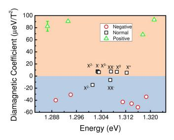
**Figure 4** Diamagnetic coefficients of different charge states in a coupled system at a pumping power of 11.85  $\mu$ W and a bias voltage of +0.5 V. The values for  $X^0$  and  $X^+$  are extracted from the spectra corresponding to a pumping power of 5.93  $\mu$ W and a bias voltage of -0.5 V, as shown in Fig. S2 in the ESM. A typical error bar for a PL peak is shown at 1.2866 eV.
