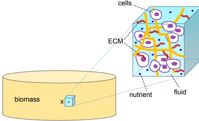
FIGURE 3. A schematic view of the computational domain  $\Omega$  with a detailed view of a typical REV where the various phases and components of the growing mixture are identified.
