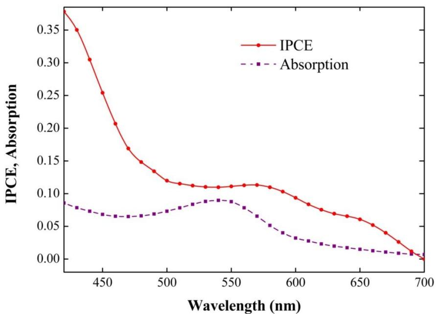
Fig. 4. Comparison of the absorption spectra of Jamun dye extract and IPCE of the Jamun adsorbed on  $\text{TiO}_2$  as in the Dye Sensitized Solar Cell.
