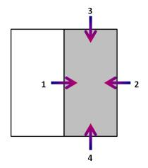
Fig 5. Temperature Gradients on a Horizontal Vane. The white (cold) side of the vane is assumed to have a temperature similar to ambient temperature and the grey (hot) side is warmer than ambient temperature.
