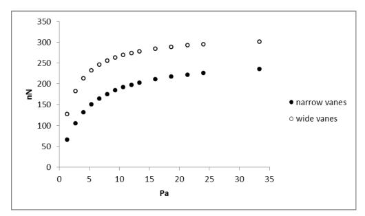
Fig 7. Drag Force at 10 rad/s (theory). The narrow vanes are 8mm by 16mm and the wide vanes are 16mm by 16mm. Both vanes have a 4mm stem connecting them to the spindle axis. The accommodation coefficient is 0.6.
