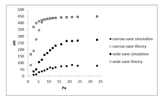
Fig 13. Thermal Creep Force (simulation and theory). The narrow vanes are 8mm by 16mm and the wide vanes are 16mm by 16mm. The temperature difference on the vanes is 9K. The characteristic length of the temperature gradient on the surface is 3.5mm. The accommodation coefficient is 0.6. Positive force is directed from the hot side to the cold side.
