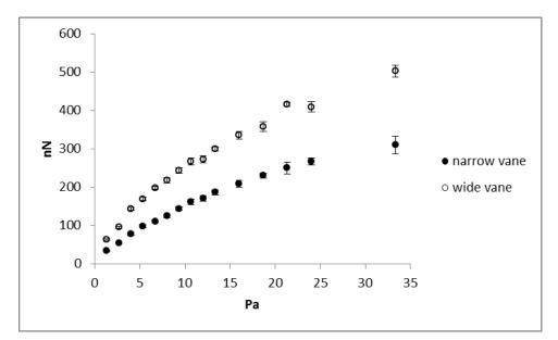
Fig 11. Drag Force at 10 rad/s (simulation). The narrow vane is 8mm by 16mm and the wide vane is 16mm by 16mm. Particle-surface collisions are calculated as if the vane is rotating about a point 4mm beyond its edge. The accommodation coefficient is 0.6. The range bars are the length of the standard deviation of the 10 segments of the trial at the reported pressure. Range bars that are not visible are hidden behind the identifying symbol.
