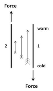
Fig. 2. Hettner Radiometer. Plate 1 has a temperature gradient and plate 2 has a uniform temperature. The temperature gradient establishes thermal creep (arrows with fletchings).
