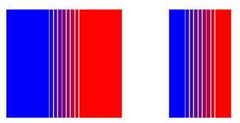
Fig. 9. Vanes as Modeled in SPARTA. The wide and narrow vanes are each divided into nine segments separated by two Angstroms. Each segment has a single assigned temperature which differs from the other segments.
