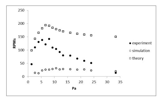
Fig. 15. Narrow Vane Angular Speed (experiment, simulation, and theory). The vanes are 8mm by 16mm. The radiometer has 4 vanes attached to the spindle by 4mm stems. The temperature difference on the vanes is 9K. The characteristic length of the temperature gradient on the vanes is 3.5mm. Positive angular speed represents rotation with the cold side leading.
