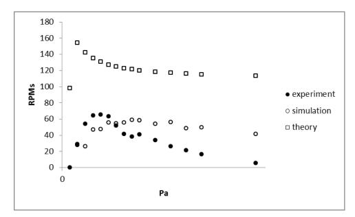
Fig 16. Wide Vane Angular Speed (experiment, simulation, and theory). The vanes are 16mm by 16mm. The radiometer has 4 vanes attached to the spindle by 4mm stems. The temperature difference on the vanes is 9K. The characteristic length of the temperature gradient on the vanes is 3.5mm. Positive angular speed represents rotation with the cold side leading.
