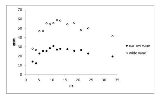
Fig 12. Angular Speed (simulation). The narrow vane is 8mm by 16mm and the wide vane is 16mm by 16mm. Both vanes have a 4mm stem connecting them to the spindle axis. The temperature difference on both vanes is 9K. The characteristic length of the temperature gradient on the surface is 3.5mm. The accommodation coefficient is 0.6. Positive angular speed represents rotation with the cold side leading.
