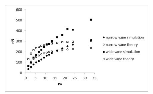
Fig. 14. Drag Force (simulation and theory). The narrow vanes are 8mm by 16mm and the wide vanes are 16mm by 16mm. The vanes have a 4mm stem connecting them to the spindle axis. They are rotating at 10 rad/s. The accommodation coefficient is 0.6.
