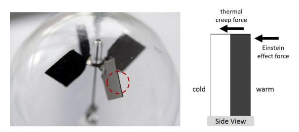
Fig 1. Motive forces on the vane of a Crookes radiometer. The figure on the right is an edge view of the vane and not to scale. In commercial Crookes radiometers, typical vanes are 1.5 cm x 1.5 cm and thickness is usually on the order of 0.1mm. The thermal creep force acts on the edge parallel to the temperature gradient. The Einstein effect acts on the surfaces perpendicular to the temperature gradient.
