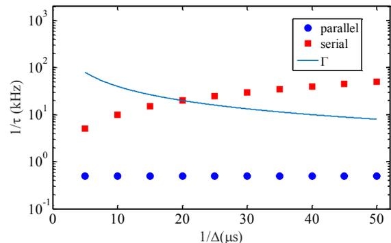
FIG. 3. Fourier limitation  $1/\tau$  as a function of AFC echo time  $1/\Delta$ , for the serial and parallel sequences discussed in section II. The target AFC peak width  $\Gamma$  is also plotted to illustrate the condition in Eq. (10).
