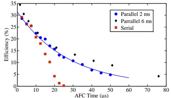
FIG. 6. AFC echo efficiency versus  $1/\Delta$  using the serial method (red squares) and parallel method with  $T_{prep} = 2$  and 6 ms (blue circles and black diamonds). For the parallel method with  $T_{prep} = 2$  ms the efficiency is fitted to an exponential decay (blue line) with a time constant of  $27.5 \mu$ s at  $\exp(-1)$  of the maximum value. For the case  $T_{prep} = 6$  ms the decay is non-exponential.
