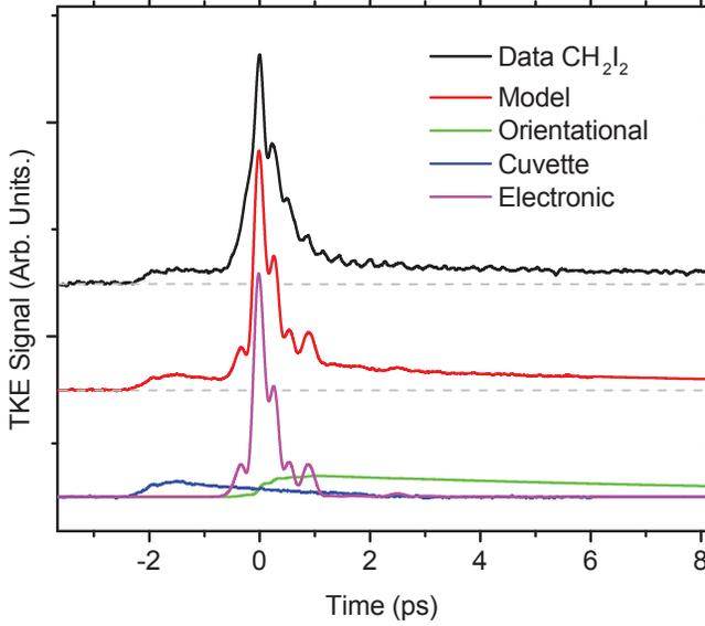
FIG. 3. Modeling of the HD-TKE signal. The experimental data for  $\text{CH}_2\text{I}_2$  are plotted at the top in black. The complete model is plotted directly below in red. The individual components of the fit, cuvette (blue), orientational (green), and electronic (magenta), are plotted together on the final line.
