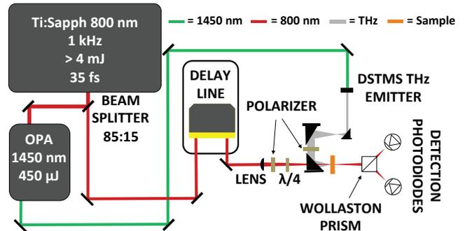
FIG. 1. The heterodyne-detected THz Kerr effect spectrometer used for THz-THz-Raman experiments. Note that the 800 nm probe beam is s-polarized and that the THz polarizer is set at  $45^\circ$  with respect to that polarization.
