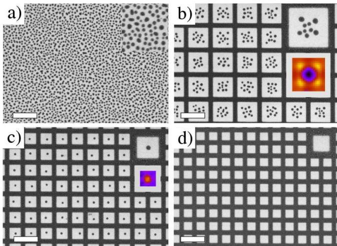
FIG. 1. SEM images of NPB deposited on a) bare, b)  $4.0\mu\text{m}$  c)  $2.2\mu\text{m}$  and d)  $1.8\mu\text{m}$  Au grid patterned  $\text{SiO}_2$  surface; inset: magnied view and in b) and c) the corresponding color coded island size distribution from the simulations (yellow high, black low value). The scale bar here is  $5\mu\text{m}$ .
