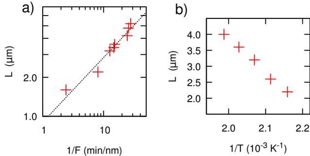
FIG. 5. Dependence of Au grid size of one NPB island in the cell on a) double logarithmic plot of beam flux at substrate temperature of  $200^\circ\text{C}$  with straight line of the slope  $1/2$  and b) substrate temperature at beam flux of  $0.12 \text{ nm/min}$ .
