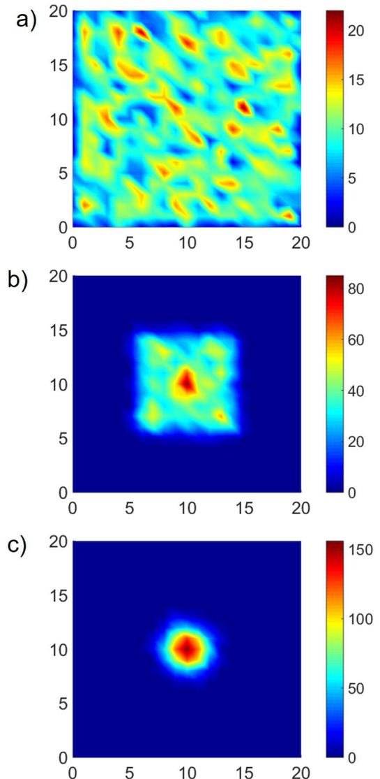
FIG. 2. Histogram of NPB islands position distribution in a)  $2.2\mu\text{m}$  grid artificially added on bare  $\text{SiO}_2$ , for comparison, b)  $4.0\mu\text{m}$  Au grid and c)  $2.2\mu\text{m}$  Au grid.
