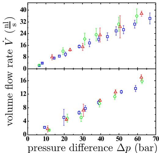
Figure 7. (Color online) Volume flow rates  $\dot{V}$  of n-hexane in V10 (upper panel) and V5 (lower panel) as a function of the applied external pressure difference  $\Delta p$  at three different temperatures: 25 °C (squares), 40 °C (circle), and 50 °C (triangle).
