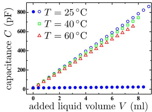
Figure 4. (Color online) Calibration measurements of the cylindrical capacitor for water (open symbols) and n-hexane (filled symbols) at selected temperatures. The capacitance  $C$  was measured as a function of the liquid amount  $V$  filled into the capacitor. For the empty capacitor it is  $C \approx 15$  pF.
