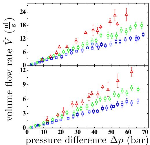
Figure 6. (Color online) Volume flow rates  $\dot{V}$  of water in V10 (upper panel) and V5 (lower panel) as a function of the applied external pressure difference  $\Delta p$  at three different temperatures:  $25^\circ\text{C}$  (square),  $40^\circ\text{C}$  (circle), and  $60^\circ\text{C}$  (triangle).
