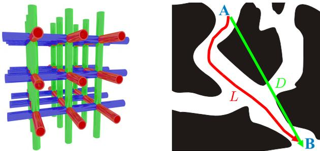
Figure 1. (Color online) Illustration of the meaning of the tortuosity  $\tau$  of a pore network such as Vycor<sup>®</sup>. (left): For an isotropic distribution of the pores only every third pore is subjected to the pressure gradient yielding  $\tau = 3$ . (right): For meandering pores an additional factor of  $\frac{L}{D}$  must be introduced to correct the length  $D$  of the direct interconnection of two points for the actual path length  $L$ .
