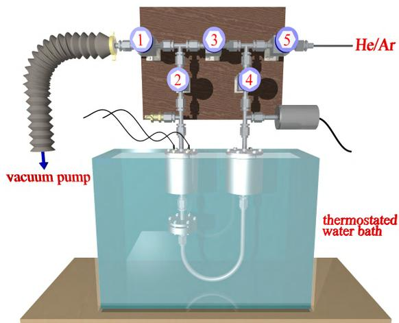
Figure 3. (Color online) Raytracing illustration of the hydraulic permeability apparatus (HPA) consisting of a gas handling and the actual flow system. The latter is temperature-controlled in a water bath. The gas handling can be evacuated by a vacuum pump and can be filled with helium or argon gas.
