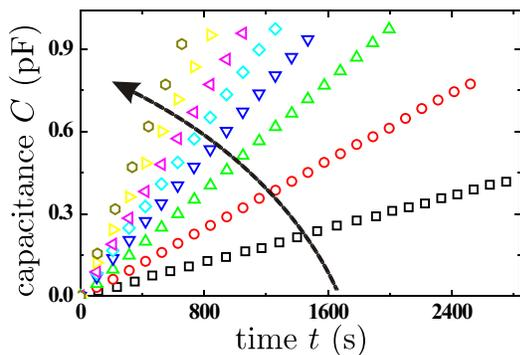
Figure 5. (Color online) Time dependent variation in the capacitance  $C$  of the cylinder capacitor due to the flow of water through V10 at  $25^\circ\text{C}$  for a series of applied external pressures. The arrow indicates the direction of increasing  $\Delta p$ . The shown measurements correspond to: 8 bar, 16 bar, 24 bar, 31 bar, 37 bar, 45 bar, 54 bar, and 70 bar. The data density is reduced by a factor of 20.
