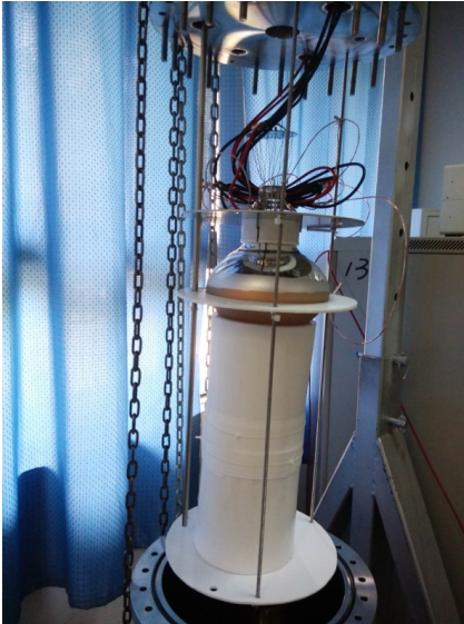
Fig. 2. The layout of LAr container and PMT.
