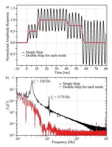
Figure 9. Amplitude response of magnetic drive. Point-to-point transitions between five amplitudes. a) Normalized response of the driving force depicted in Figure 8. Single-step forcing between levels results in significant long term ringing. A double-step for each mode results in a smooth, oscillation-free response. b) FFT of a) depicts large first and second mode amplitudes for the single-step drive. The double-step for each mode completely eliminates the frequency peaks at 320 Hz and 1179 Hz.
