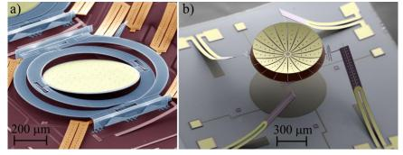
Figure 1. Two MEMS micromirrors examples. a) LambdaRouter, a commercial MEMS mirror built by Lucent Technologies. The mirror pivots around two axes and is used as the optical switching element in a large network cross-connect. Photo Courtesy of Lucent Technologies Inc. b) Varifocal mirror, driven by electrothermal bimorphs, used for beam-steering in a smart lighting application.
