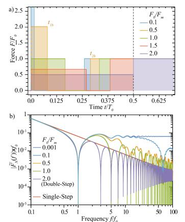
Figure 13. Actuation traces and their Fourier transforms of Overdrive b. a) Five Overdrive forcing examples ranging from  $F_m = 10 \ F_0$  to  $F_m = F_0/2$ . b) Fourier transform of Overdrive b drive force. As is the case for Overdrive a, the resonant mode can be suppressed from any drive force. The shorter time pulses for increased  $F_m$  result in higher actuation forces acting at higher frequencies.
