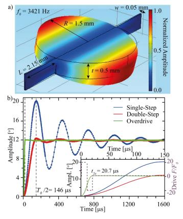
Figure 12. Simulation of a single-axis mirror. a) The fundamental torsional mode appears at 3421 Hz. b) Single-(blue), double-step (red), and Overdrive (green) actuation. The Overdrive results in a settling time seven times faster compared to the double-step actuation and is completed after only  $t_{2a} = 20.5 \ \mu s = To/14.3 \ for \ F_m = 20 \ F_o$ .
