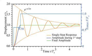
Figure 3. Single- and double-step response of a dissipative resonator.  $(\gamma = 0.2)$  results in the rather rapid decay of the single step response. The duration of the first step of the double-step forcing scheme is very close to  $T_0/2$ , while the forcing must be raised to  $0.58 \times F_0$ , where  $F_0 = k x_0$  is the steady state force required to reach  $x_0$ .
