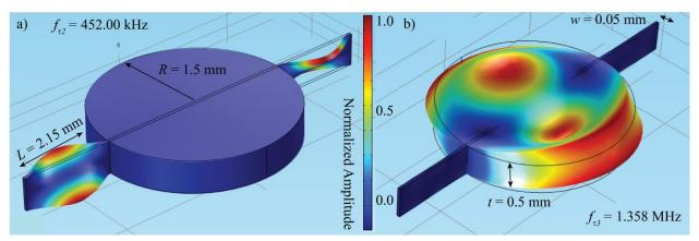
Figure S2. Finite element simulation of single axis mirror. The higher order torsion modes occur at a)  $f_{\tau 2} = 452$  kHz and b)  $f_{\tau 3} = 1.3558$  MHz, where the fundamental torsion mode (Fig. 15a)) has a resonance frequency of  $f_{\tau l} = 320$  Hz.
