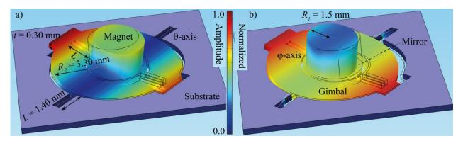
Figure S1. Finite element simulation of a dual axis mirror with a magnet attached. Color indicates normalized displacement. a) The fundamental torsional mode was found experimentally at 320 Hz. b) The higher order mode, also actuated by the externally applied torque, experimentally found at 1179 Hz. This mode is the planar flexural mode, where the tilt results from the asymmetry caused by the magnet. These two modes couple when a step in the force is applied.
