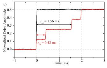
Figure 8. Magnetic drive transduction. Two modes couple into the step function. a) Normalized drive of single-step and two double-step actuation schemes, for switching between five amplitudes. b) First transition from 0 to 50 % of the maximum amplitude. Each transition of the double-step is split into two to account for both modes.
