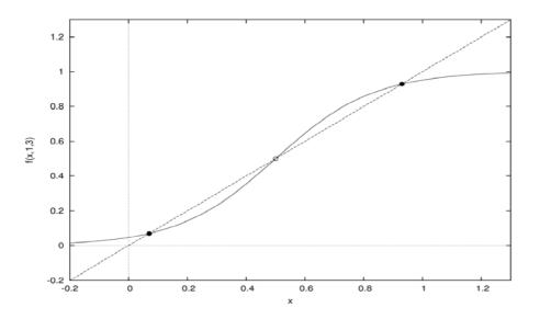
Figure 3: The activation function for the basic system with  $\theta = 1$  and a = 3. Filled and empty dots represent stable and unstable fixed points, respectively.
