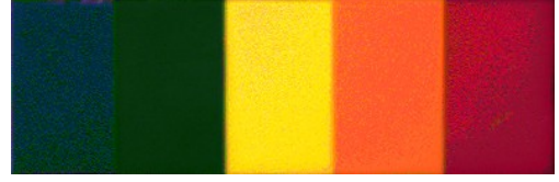
Fig. 3. The icon used for real-world testing in the second set of experiments. The true reflectance spectrum was measured for each unique section of the icon and then compared to the predicted spectra from the three inverse methods.
