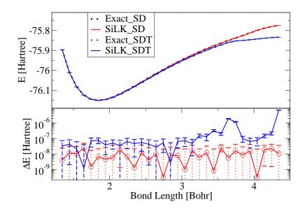
FIG. 5. Potential energy curves for H<sub>2</sub>O molecule using the DZ basis and the SD and SDT vector spaces. The exact results obtained from exact diagonalization and the SiLK results are shown.  $P = 2 \times 10^{10}$  is used for all the bond lengths in the SD and the SDT vector spaces.
