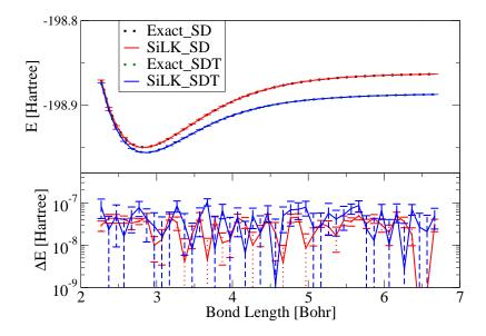
FIG. 8. Potential energy curves for  $F_2$  molecule as a function of bond length and using the Hartree-Fock determinant plus either the SD and SDT vector spaces. The exact results obtained from exact diagonalization and the SiLK results are shown.  $P = 2 \times 10^{10}$  is used.
