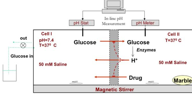
FIG. 2.1. *Diagram of the Experimental Oscillator [2, 15]*
