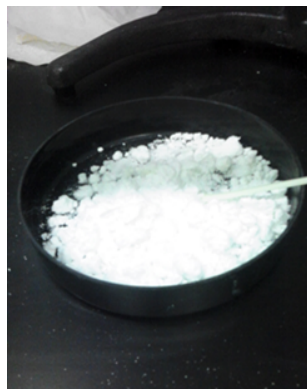
Figure 7.11: Ammonium molybdate obtained from the recovery of \text{CaMoO}_4 crystals.
