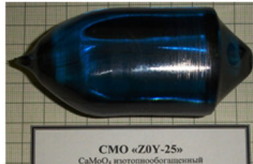
Figure 3.14: ^{48\text{depl}}\text{Ca}^{100}\text{MoO}_4 crystals grown at the Innovation Center of the Moscow Steel and Alloy Institute (ICMSAI) in Russia.
