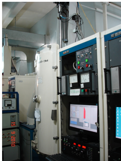
Figure 3.2: A photograph of a CRYSTAL-3M Crystal puller (at JSC Fomos-Materials).
