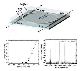
Figure 1. Top: Hydex based micro-ring resonator with Q factor of 1.2M. Bottom: Spectra of hyper-parametric oscillator at full pumping power (101mW, right). Output power of a single line, single port vs pump power (bottom, left).
