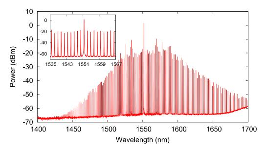
Fig. 4. Spectrum of the comb generated from the microring, measured by an OSA with a resolution of 0.5nm. Inset: Zoom-in of the spectrum around the pump wavelength.
