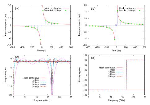
Fig. 2. Working principle of a transversal Hilbert transformer: (a) - (b) Ideal, continuous hyperbolic and discretely sampled impulse response with time spacing  $\Delta t = 59$  ps. Corresponding (c) amplitude and (d) phase response for the continuous and discrete cases, respectively.
