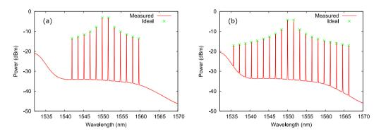
Fig. 5. EDFA2 output showing the weight of each tap for: (a) 12 tap filter, and (b) 20 tap filter
