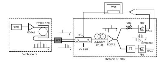
Fig. 3. System implementation of a Hilbert transformer exploiting a microring-based comb source. VNA is a Vector Network Analyzer, WS= wavelength selective switch, VOL=variable optical attenuator.
