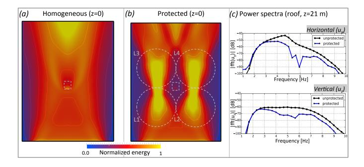
FIG. 3. (a) Maps of the elastic energy distribution at the surface (z=0) for the homogenous case. Same as (b) but for the lenses case. (c) Spectral density of the rooftop motion of the building in dB. The blue trace is calculated for the homogeneous case while the black is obtained when the lenses enclose the building. (d) same as a (c) but for the vertical component.
