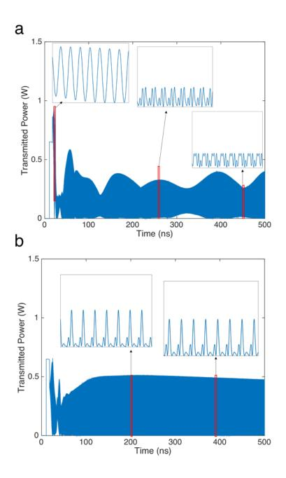
FIG. 3. Temporal output of 38 cm-long chalcogenide fiber Fabry-Perot cavity for a 500-ns pulse input and two different values of phase shift. a)  $\Delta \phi_0 = 1.8\pi$  b)  $\Delta \phi_0 = 0.62\pi$
