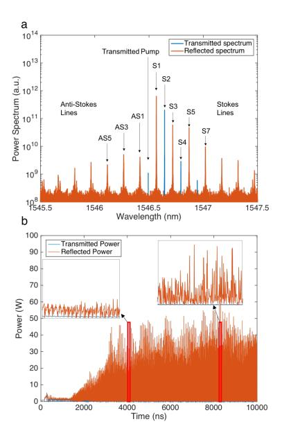
FIG. 2. (a) Output spectrum of a silica fiber ring cavity with feedback of 99% of the backward Stokes. The odd-order Stokes and ant-Stokes lines are spaced by twice the Brillouin frequency. (b) Temporal output showing erratic pulsations.
