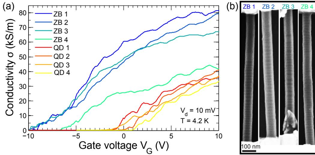
FIG. A.1: (Color online) (a) Conductivity as a function of gate voltage for four reference ZB segments (blue-green color scale) and for four QD devices (red-yellow color scale). (b) SEM images of the ZB reference devices optimized to observe the twinned segments.
