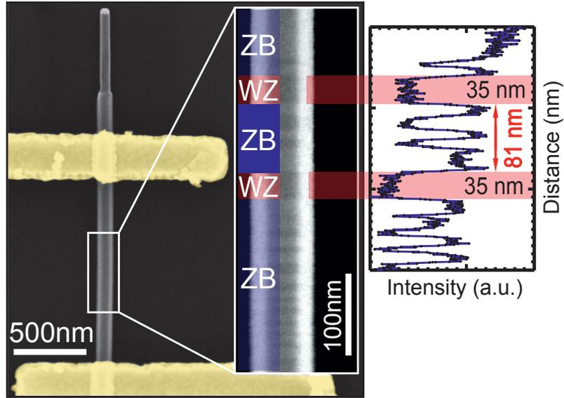
FIG. A.3: (Color online) (a) SEM images from Fig. 4(f) in the main text with (b) corresponding intensity profile.
