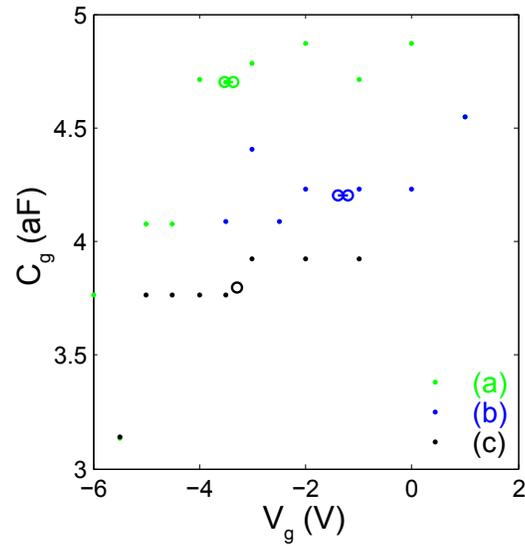
FIG. A.4: (Color online) Gate capacitance as a function of gate voltage. Results from fast Fourier transform (FFT) analysis (dots) where the gate sweep has been divided into subintervals when performing FFT; the point in the graph indicates the start of one such interval. The circles indicate from which gate-voltage range the  $C_g$  displayed in Fig. 5 are extracted.
