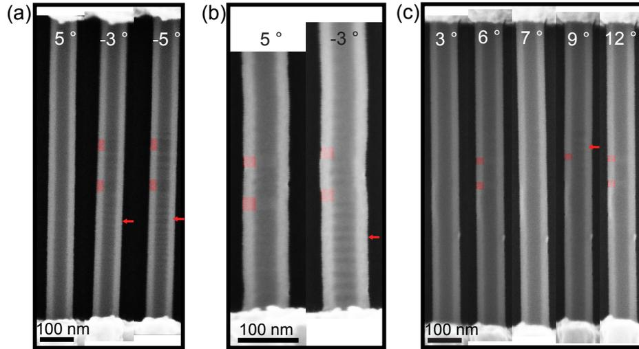
FIG. A.2: (Color online) (a)-(c) SEM images of three different QD devices at different tilt angles of the SEM stage. When visible, the WZ segments are colored red, and tilt angles where twinned segments in ZB are visible are indicated by arrows.
