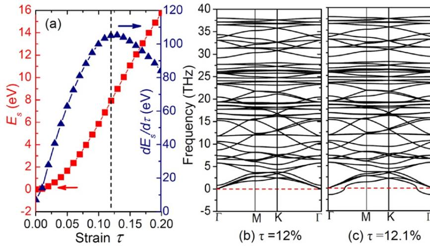
Figure 4. (a) Variation of energy in response to tensile strain. (b)-(c) Phonon spectra of g-C<sub>2</sub>N under the biaxial tensile strains of 12% and 12.1%. The negative frequencies correspond to the imaginary frequency modes which are dynamically unstable.
