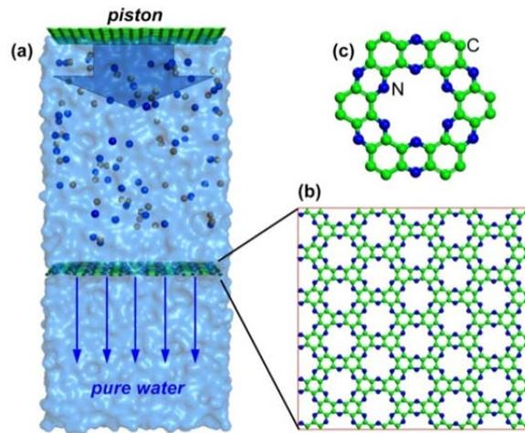
**Figure 1.**(a) Illustration of the simulation model; (b) Top view of the nanoporous g-C<sub>2</sub>N layer; (c) Local structure of one nanopore in g-C<sub>2</sub>N.
