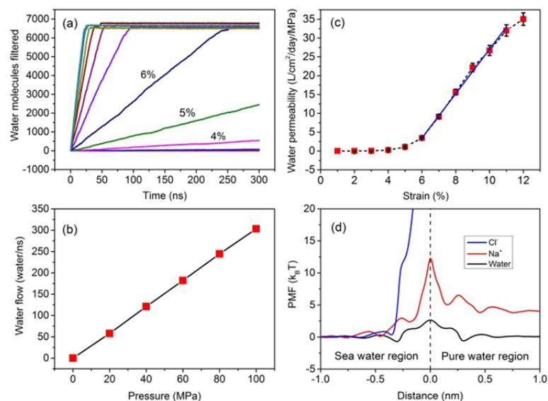
**Figure 2.** (a) Number of water filtered by g-C<sub>2</sub>N membrane as a function of simulation time under piston pressure of 100 MPa, (b) Water flow at various pressure through the 12%-stretched g-C<sub>2</sub>N, (c) Water permeability with respect to tensile strain and (d) Potential of mean force (PMF) of water, Na<sup>+</sup> and Cl<sup>-</sup> passing through the 12%-stretched g-C<sub>2</sub>N filter from seawater region to pure water region. The filter is placed at 0 nm.
