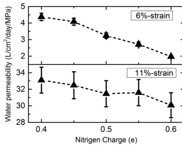
**Figure 3.** Water permeability with respect to the charges of nitrogen in the g-C<sub>2</sub>N filter under tensile strain of 6% and 11%.
