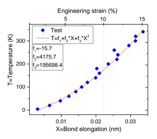
**Figure 6.** Curve of temperature v.s. maximal bond elongation due to thermal vibration of atoms on SLBP. Temperature varies in [4.3, 340] K.
