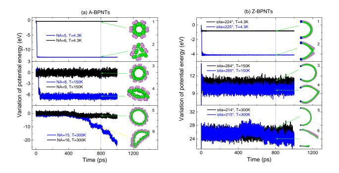
**Figure 2.** Variation histories of potential energy of curved SLBPs along different direction at different environmental temperatures, e.g, 4.3, 150 and 300K: (a) along armchair direction, the A-BPNTs are formed with chirality of ( $N_A$ , 7, 360 °); (b) along zigzag direction, the Z-BPNTs are formed with partial chirality of (6, 15,  $\theta$ /sita) at 4.3K or (6, 31,  $\theta$ ) at 150 and 300K. The snapshots of related (axial view) models at 800 ps are inserted.
