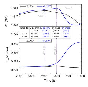
**Figure 5.** Histories of  $\alpha$ 1 and L\_bc (=L<sub>bc</sub>) of the structure under critical states at 4.3 K.
