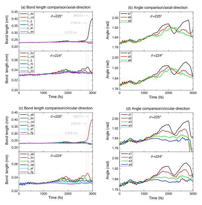
Figure 4. Histories of bond angles and bond lengths in the Z-BPNTs of  $(6, 15, \theta)$  at 4.3 K with different curved
