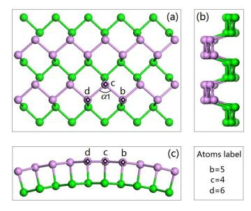
**Figure 7.** Three-view of a segment of a Z-BPNT. The three (purple) atoms, i.e., b( or 5), c(or 4) and d(or 6), and bond angle  $\alpha$ 1 on the outer layer of tube. Letters of b, c and d represent the atoms on the BPNT, numbers of 4, 5 and 6 represents the atoms on SLBP.
