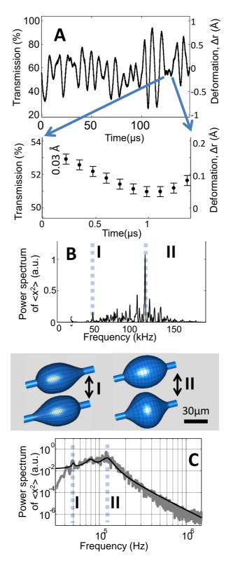
**Figure 2, Experimental results: Droplet fluctuations** are shown in the temporal (A) and frequency domains (B) where the oscillation frequencies that dominate over their vicinity are linked to calculated droplets modes (Supplementary movie 1-2) (inset). The blue arrows lead to a zoom-in plot where each of the points represents the transmission average over a 125 ns period. The error bar represents the standard deviation for each averaging. Presenting the
