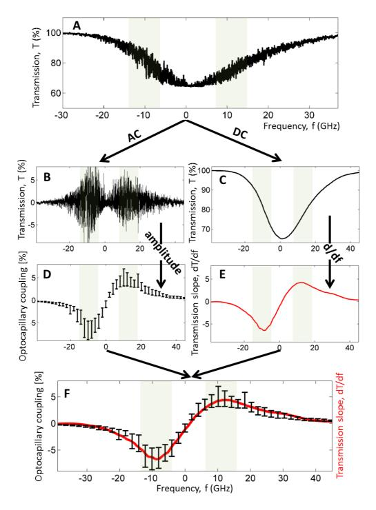
**Figure 3, Experimentally reaching maximal optocapillary coupling** at the region where the optical resonance has the steepest transmission slope. Slowly scanning the laser frequency
