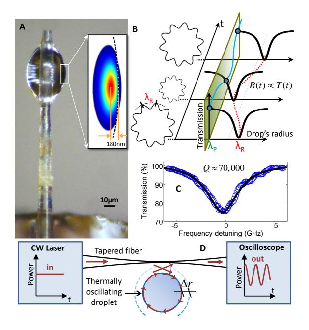
**Figure 1: Experimental setup:** (A) Micrograph of the water µdroplet along with its calculated fundamental optical mode shape (inset). (B) A Lorentzian transfer function (black) converts radius drifts (red) into changes in optical transmission (blue). (C) Monitoring droplet resonator transmission while scanning a wavelength through resonance reveals its optical quality factor. (D) Experimental setup scheme. Laser wavelength is 980 nm.
