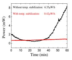
Fig. 7. Power stability in OFF state for 1 h with (red solid line) and without temperature stabilization (black solid line).
