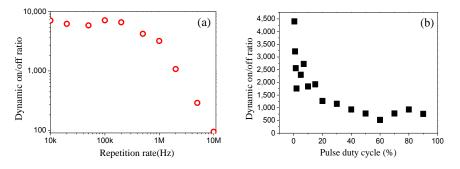
**Fig. 6.** (a) Dynamic on/off ratio at 5 ns pulse duration versus laser pulse repetition rate. (b) Dynamic on/off ratio versus laser pulse duty cycle atrepetition rate of 1
