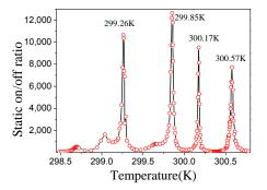
Fig. 5. Measured static on/off ratio of MZ-EOIM at different temperatures.
