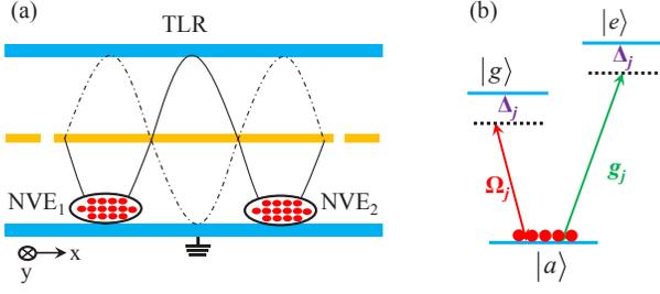
FIG. 3: (a) Schematic diagram of the hybrid quantum system, which consists of two NVEs coupled to a high-Q TLR. (b) The  $V$ -type energy-level configuration for the ground state of NVE driven by the resonator and appropriate external magnetic fields.
