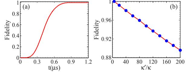
FIG. 4: (a) Fidelity of the population transfer scheme with MSDs from  $|\phi_2\rangle = |0eg\rangle$  to  $|\phi_1\rangle = |0ge\rangle$  under the influence of dissipations. In the simulation,  $\kappa^{-1} = 50 \mu\text{s}$  [32],  $\gamma^{-1} = 6$  ms,  $\gamma_\varphi^{-1} = 600 \mu\text{s}$  [33], and other parameters are the same as those for Fig. 1(c). (b) Fidelity of the population transfer scheme with MSDs for different cavity decay rates  $\kappa'$  (in units of  $\kappa$ ).
