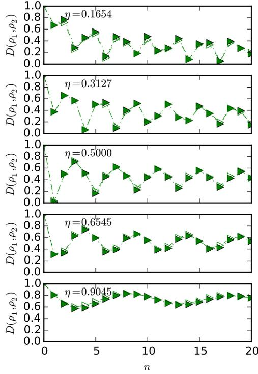
Fig. 4. Trace distance dynamics for different values of  $\eta$  for parameters  $\Delta n = 0.008995$ , FWHM = 6 nm,  $\lambda = 800$  nm and  $\Delta L = 120\lambda$ . Initial state pair is  $|H\rangle, |V\rangle$ . Filled markers are for the experimental data and empty markers are for the theoretical calculation.
