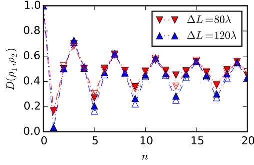
Fig. 2. Trace distance dynamics for two different quartz plate thicknesses  $\Delta L$  for parameters  $\Delta n = 0.008995$ , FWHM = 6 nm,  $\lambda = 800$  nm and  $\eta = 0.5$ . Initial state pair is  $|H\rangle$ ,  $|V\rangle$ . Filled markers are for experimental results and empty markers are for numerical simulations.
