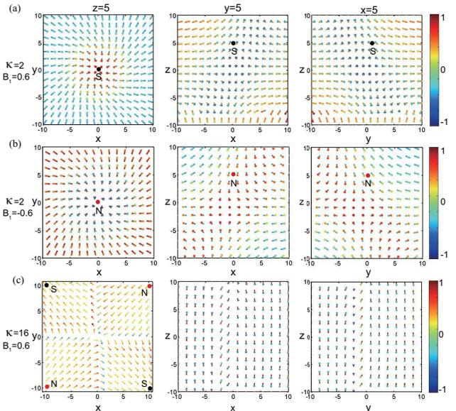
FIG. 4: (Color online). (a) Spin textures of M-PCV describe the south magnetic poles (the black dot S). (b) Spin textures of the antimonopoles describe the north magnetic poles (the red dot N). (c) Spin textures of M-SL represent spin configurations of the south magnetic poles (the black dot S) and north magnetic poles (the red dot N). Other parameters are same as in Fig.1.
