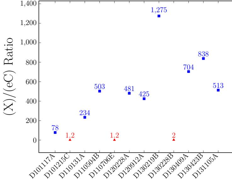
**FIG. 5.** (X) vs. (eC) peak intensity ratios of MDSI structures grown with Ga4 and Ga8, respectively. This ratio increases roughly with time if Ga4 (blue dots) is used, but remains very small with Ga8 (red triangles).
