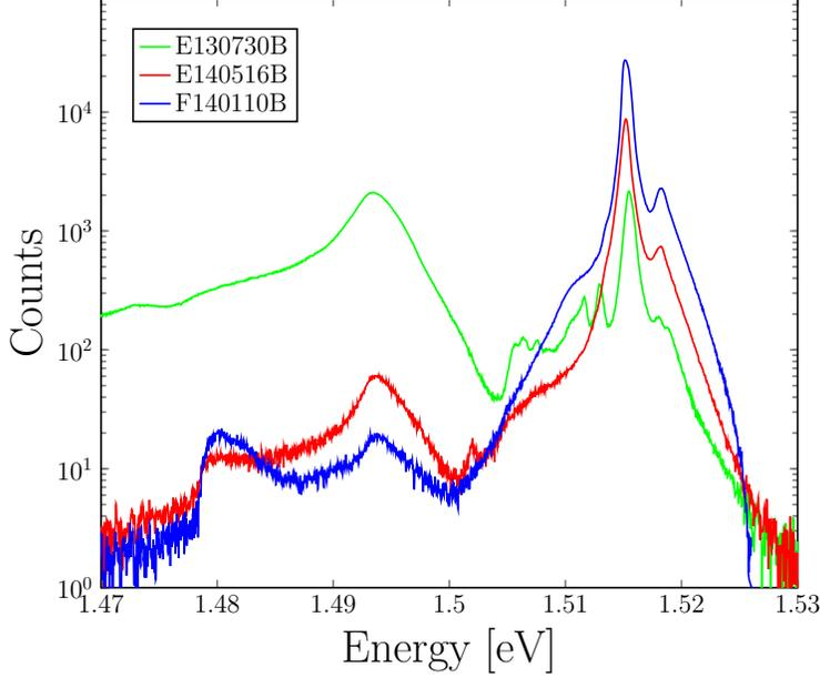
**FIG. 7.** PL spectra of wafers grown in two other MBE systems. The spectra shown in blue and red correspond to samples with reasonably high mobilities. The mobility of one in green is only  $0.23 \cdot 10^6 \text{ cm}^2/\text{Vs}$ .
