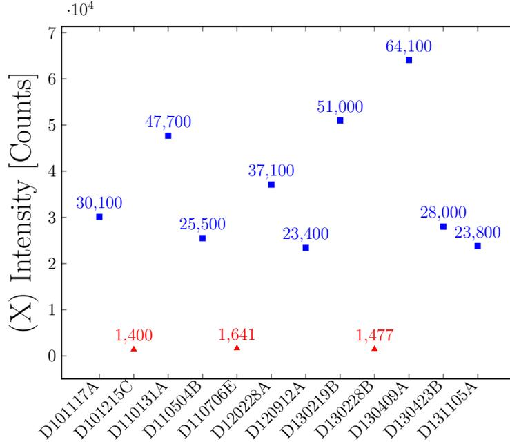
**FIG. 4. Comparison of the exciton PL intensity for several wafers from one growth campaign. The samples marked with red triangles were grown with Ga8 , the other ones (blue squares) with Ga4.**
