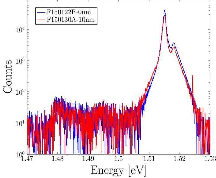
FIG. 9. PL data of a standard wafer and of one where Al impurities at 10 nm from the interface have been added to the GaAs. Although the electron mobilities of the two samples differ by more than a factor of 10, the PL spectra are very similar.
