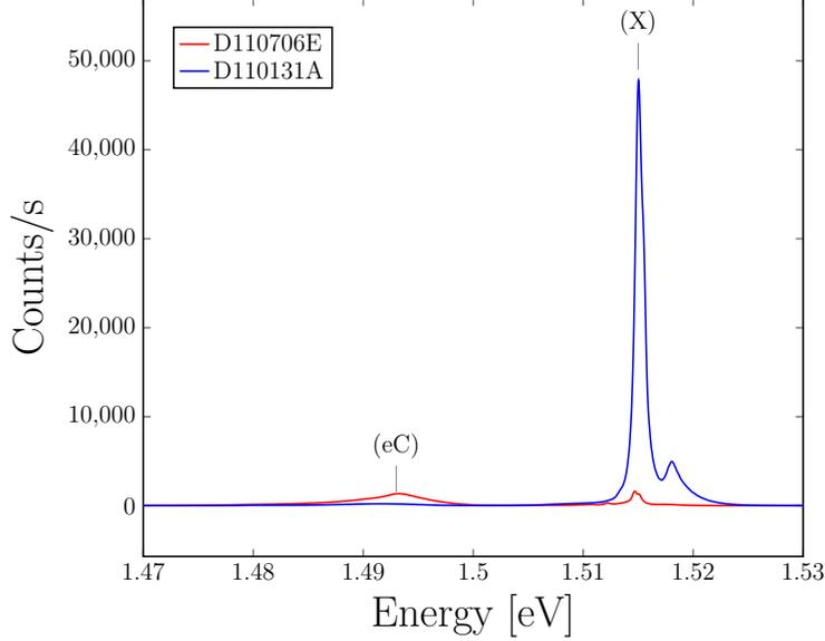
**FIG. 2.** GaAs spectra of two MDSI samples grown in the same chamber with two different gallium cells (blue: *Ga4* D110131A, red: *Ga8* D110706E). The only difference between the growth procedures of the two wafers is the choice of the gallium.
