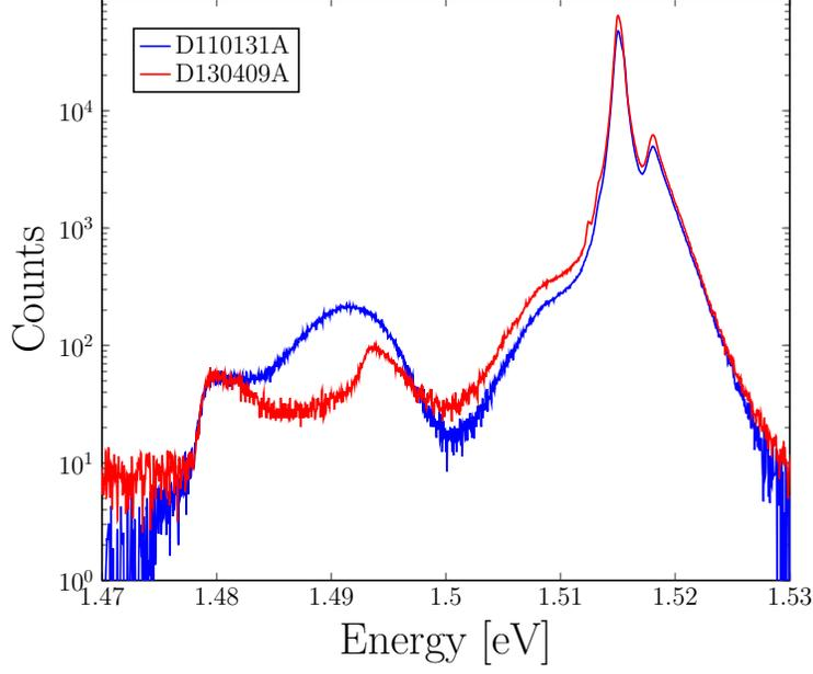
FIG. 6. PL spectra of two wafers grown about two years apart using the same "good" gallium lot Ga4. The main change over this very long growth period is the reduction of the acceptor related luminescence.
