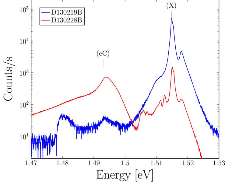
**FIG. 3.** PL spectra of the samples D130219B (*Ga4*) and D130228B (*Ga8*) which are produced in the same growth campaign as those of Fig. 2 but about two years later. The large discrepancy between the two samples in the (X) vs. (eC) ratio is nearly unchanged.
