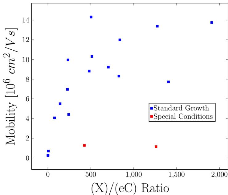
FIG. 8. A plot of electron mobility vs. the  $(X)/(eC)$  ratio shows a correlation between the two quantities for many samples.
