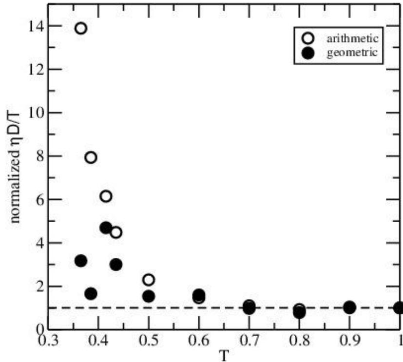
**Figure 3.** The quantity  $\eta D/T$  is plotted against  $T$  using the diffusion constants for the A particles obtained by arithmetic and geometric averaging, as indicated. To clarify the high temperature Stokes-Einstein behaviour,  $\eta D/T$  has been normalized in each case so that the high  $T$  limit is set to one with a horizontal dashed line included as a guide to the eye.
