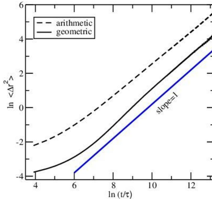
**Figure 2.** The log-log plot of the mean squared displacement  $\langle \Delta r^2 \rangle$  vs time of the A particles for the binary mixture at  $T = 0.415$  calculated as the arithmetic and geometric mean. Both curves reach an asymptotic slope of one, consistent with Fickian diffusion, but with different diffusion constants.
