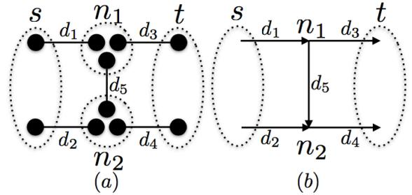
Fig. 1. (a) A repeater network with four vertices (a source  $s$ , a sink  $t$  and two nodes  $n_1, n_2$ ) and five edges (each associated with a maximal entangled state of dimension  $d_i$ ). (b) A corresponding quantum network with a directed graph. The directed edges represent noiseless quantum channels.
