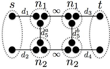
Fig. 3. An equivalent repeater network of Fig. 1(a) with  $d_5^a d_5^b = d_5$ . Each node ( $n_1$  or  $n_2$ ) is split into two nodes that are connected by a maximally entangled state with infinite dimension. The left two nodes of  $n_1$  and  $n_2$  are connected by a maximally entangled state with dimension  $d_5^a$ . The right two nodes of  $n_1$  and  $n_2$  are connected by a maximally entangled state with dimension  $d_5^b$ .
