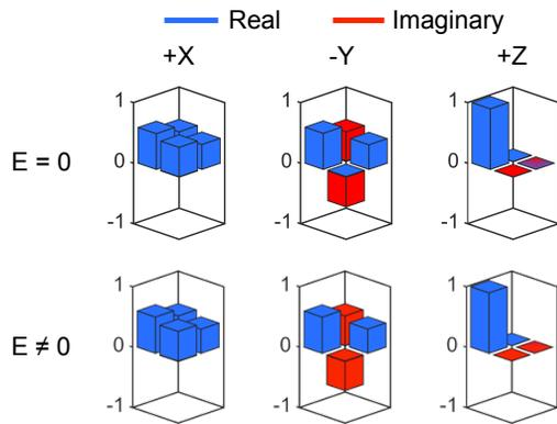
FIG. 3. SEMM output density matrices with or without electric field in  $^{151}\text{Eu}^{3+}:\text{Y}_2\text{SiO}_5$  determined by quantum state tomography. The average fidelity over  $\pm X, \pm Y$  and  $+Z$  input states is 0.999.
