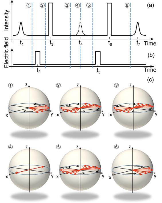
FIG. 1. The SEMM sequence. (a) microwave or optical fields. The memory input is at  $t_1$ ,  $\pi$  pulses at  $t_3$  and  $t_6$ , and the output at  $t_7$ . (b) electric field. The Stark pulses at  $t_2$  and  $t_5$  produce a phase shift that cancels the collective emission at  $t_4$ . (c) Bloch sphere representations of the wavepackets evolution at the points labeled in (a) and (b). For clarity, the input pulse has an  $\pi/2$  area.
