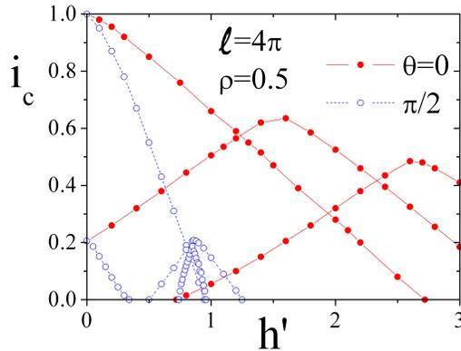
FIG. 3. (Color online) Numerical magnetic diffraction patterns,  $i_c(h')$ , of a long CAJTJ with  $\ell = 4\pi$ ,  $\rho = 0.5$  and  $n = 0$  for two values of the in-plane field orientation,  $\theta = 0$  and  $\pi$ . The magnetic field is normalized to  $J_c c$ .
