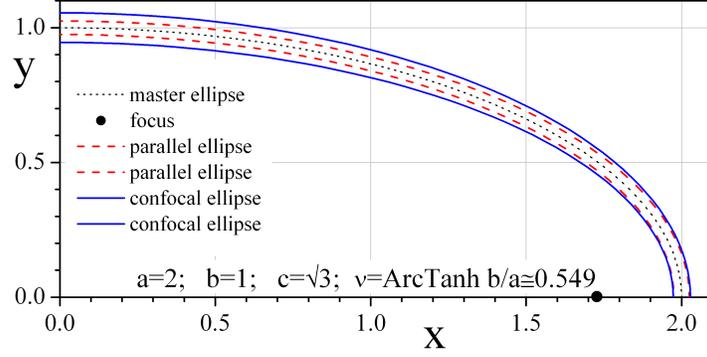
FIG. 1. (Color online) Illustration of the difference between a confocal annulus delimited by the two confocal ellipses (blue solid lines) and an elliptic annulus bounded by the two *parallel* ellipses (red dashed lines). The *parallel* ellipses are not ellipses - see Eqs.(2) and (3).
