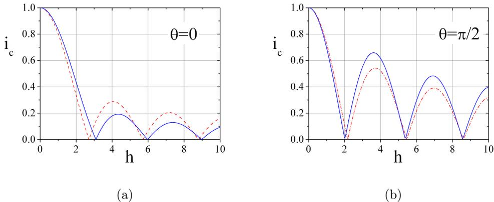
FIG. 2. Comparison of the MDPs of a small and narrow confocal (blue solid line) and elliptic (red dashed line) annular junction having  $\rho = 0.5$  and  $n = 0$  for two orientations of the applied in-plane magnetic field: (a)  $\bar{\theta} = 0$  and (b)  $\bar{\theta} = \pi/2$ . Since  $i_c(-h) = i_c(h)$ , we only show the dependence for positive field values.
