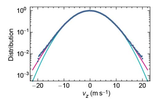
Figure 3 | Non-thermal velocity distributions. When kinematic effects of (laser-induced) chemistry are included in MD simulations, the  $\mathrm{HD}^+z$ -velocity distribution exhibits non-thermal distributions with pronounced tails (blue data points). Indeed, a least-squares fit with a q-Gaussian (magenta curve, with fitted temperature T=11.00(3) mK and q = 1.070(3) produces a visibly better result than a fit with a thermal (normal) distribution (turquoise curve, fit with T= 11.60(3) mK).
