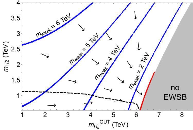
Figure 2: Contours of  $m_{weak}$  (blue) in the  $m_{H_u}$  vs.  $m_{1/2}$  plane for  $m_0 = 5$  TeV,  $A_0 = -8$  TeV,  $\tan \beta = 10$  and  $m_{H_d} = 1$  TeV. Above the black dashed contour is where  $m_h > 124$  GeV. The red region has  $m_{weak} < 0.5$  TeV. The arrows show the direction of the statistical/anthropic pull on soft SUSY breaking terms.
