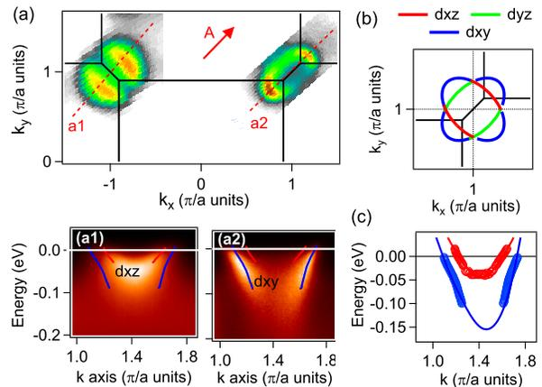
Figure 2. (a) Fermi Surface measured in Co8 at  $T=25$  K, with polarization  $A$  along the red arrow and photon energy 34 eV. (a1)-(a2) Energy-momentum images of the two different cuts indicated in (a). (b) Sketch of the orbital characters on the two electron pockets expected by calculation. (c) Experimental band dispersion (symbols) compared with calculated bands shifted and renormalized as indicated in Table 1.
