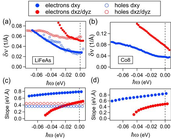
Figure 6. (a-b) MDC half width at half maximum  $\delta\nu$  as a function of binding energy in LiFeAs (a) and Co8 (b). (c-d) Slopes of the dispersion used to compute  $1/\tau$  (Eq. 3) in LiFeAs (c) and Co8 (d). For electron bands, it is the slope of the renormalized LDA dispersion. For hole bands, it is straight lines, as they give a better or equivalent fit than the LDA (see Fig. 3d).
