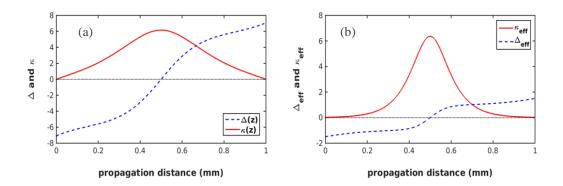
Figure 3. (color online). Spatial profile of coupling and mismatch. (a)  $\Delta(z)$  (dashed) and  $\kappa(z)$  (solid) determined through Invariant based method, (b)  $\Delta_{eff}(z)$  (dashed) and  $\kappa_{eff}(z)$  (solid) determined from transitionless driving method.
