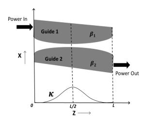
**Figure 1.** Schematic diagram for tapered waveguide coupler of length *L*. Propagation direction is along *z* direction.  $\beta_1$  and  $\beta_2$  are the propagation constants. Separation between the waveguides varies along *z* and the coupling coefficient  $\kappa$ attains a maximum at z = L/2.
