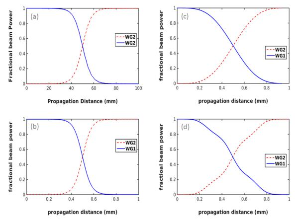
Figure 4. (color online) Spatial evolution of fractional beam power with respect to z for (a) adiabatic case with L = 100mm, (b) Transitionless driving where L = 1mm, (c) & (d) Invariant based approach using the Hamiltonian and the invariant respectively, L = 1mm.
