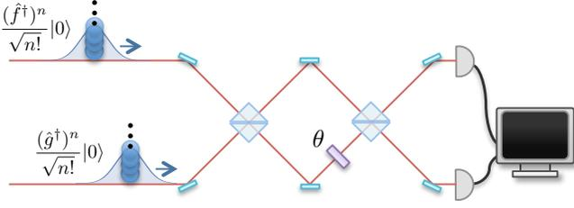
**FIG. 1. Mode-mismatch introducing photon distinguishability:** The probe state shown,  $|n\rangle_{f,1}|n\rangle_{g,2}$ , enters an Mach-Zehnder interferometer before being measured with photon number-counting measurements. The overlap of the temporal modes governs how much quantum interference occurs at the beam splitters.
