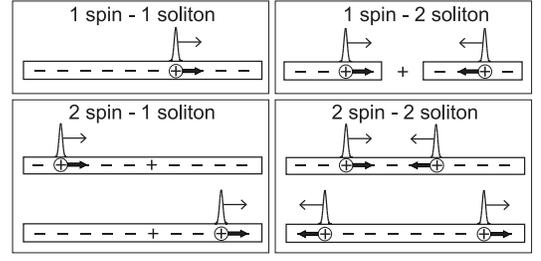
FIG. 5. Schematic pictures of spin transfer for a single soliton (left) and a double soliton (right). The flipped spins, denoted by the symbol +, follow soliton potentials. The upper (lower) panels show states in the single (double) spin-flip sector.
