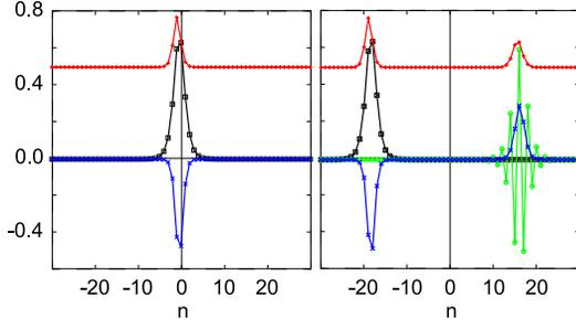
FIG. 3. (Color online). Soliton solutions to the Toda equations. for single soliton (left) and double solitons (right). Plotted are  $J_n(t)$  (red lines with +),  $h_n(t)$  (blue with  $\times$ ), the ground-state wavefunction (black with boxes), and the first excited-state wavefunction (green with circles) at a fixed  $t$ .
